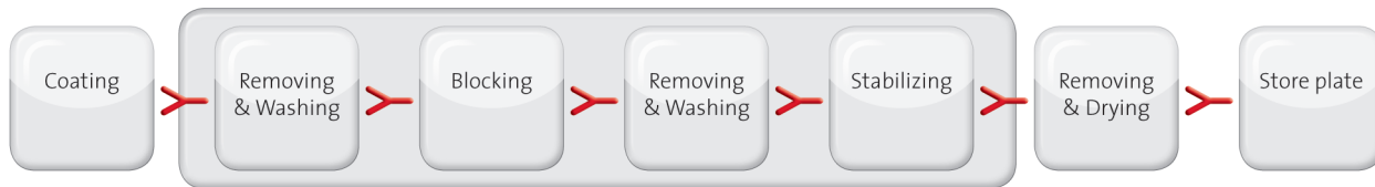
Standard plate processing
